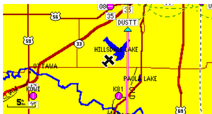
'Vectors' creates an extension of the final course, beyond the final approach fix
