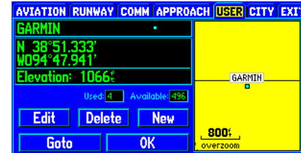
To display user waypoint information press ➔ WPT and select the 'USER' file tab.
