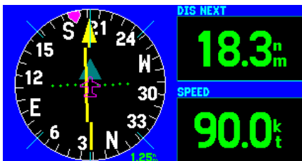
'2 Big Number Fields' displays the HSI with two large-character data fields along the right-hand side of the page.
